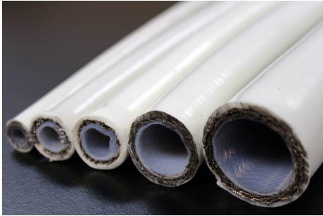
ST-Flex Smoothbore PTFE Lined SS Braided Hose with Silicone Cover (1/8" to 1" ID)
