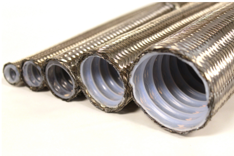
C-Flex Convoluted PTFE Lined SS Braided Hose Assemblies (3/8" to 4" ID)
